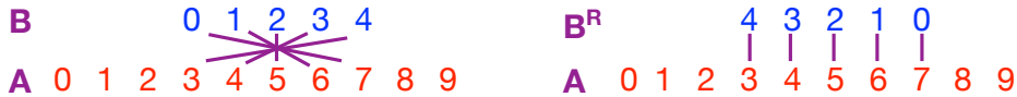
Figure 5.5: Convolution of strings becomes equivalent to string matching when the pattern is reversed.
