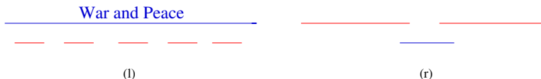
Figure 1.6: Bad instances for the (l) earliest job first and (r) shortest job first heuristics. The optimal solutions are in red.
