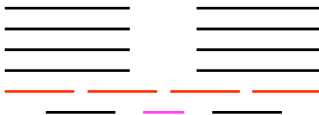
Figure 1.7: Counter-example to the greedy heuristic for movie star scheduling. Picking the pink interval, which intersects the fewest others, blocks us from the optimal solution (the four red intervals).
